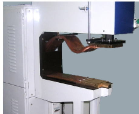
Deep Throat CD Projection Welding Machine to weld specialized sheet metal components
