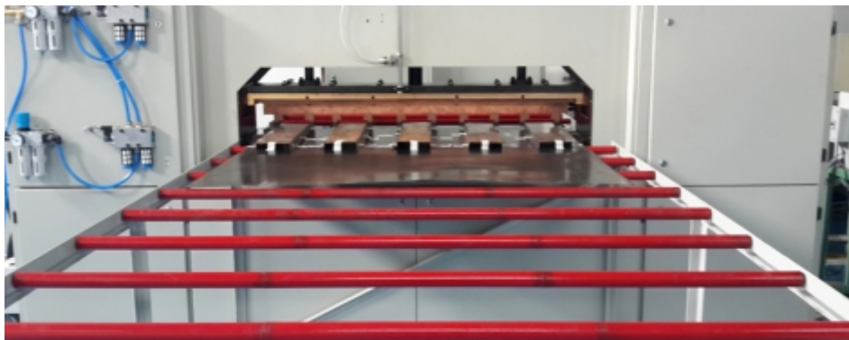
CD Projection Welding Machine with automated feeding to weld Stiffener on fire door panels
