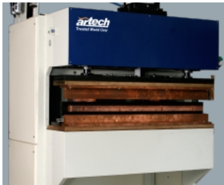
CD Projection Welding Machine with specialized electrodes to weld components in Hollow Metal Doors
